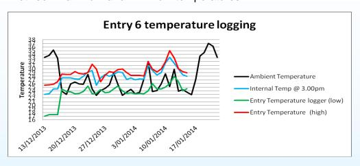
The above graph shows how the ambient temperature fluctuation is quite wide however, the difference between the low and high temperatures remain fairly consistent after the coating is supplied, reducing the high temperature and increasing the low temperature giving a more stable environment.
