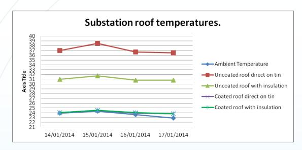
As can bee seen on this graph the temperatures show both treated and untreated surfaces, the efficiency of the coating is easily seen.
